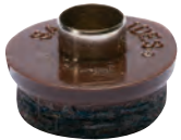
PS12 ■ 3/4" FELT BASE ■ NO DRILLING NEEDED ■ INSTALL W/ TAP OF A HAMMER ■ VERY THIN TUBULAR RIVET, HOLDS FAST AND PREVENTS SPLITTING ■ GREAT FOR END GRAIN
